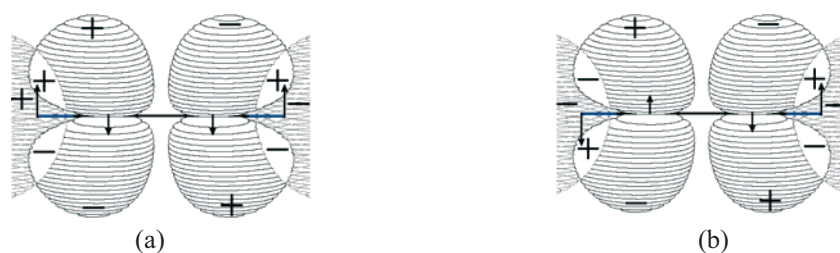
Fig. 4. Schematic illustration to the covalence origin of the vibronic instability of the linear configuration of \text{H}_2\text{O}_2 : (a) \pi_g \otimes \sigma_u , (b) \pi_g \otimes \sigma_g . The overlap integral between the vibronically mixing molecular orbitals (white areas) is zero in the linear D_{\infty h} configuration and becomes nonzero by \pi_g ( \pi_u ) distortions bending the \text{H}_2\text{O}_2 molecule towards to the cis\text{-}C_{2v} (a) and trans\text{-}C_{2h} (b) transition states
